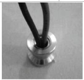
Take the threaded mushroom and screw down onto the exposed threaded rod. Pull the wire through and attach to the wire connection on the individual bar.
