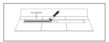
4 Apply an appropriate amount of tile adhesive or silicon to the channel cut-out.
