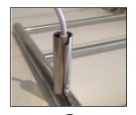
Select the leg with the cutaway and feed the cable through the leg.
